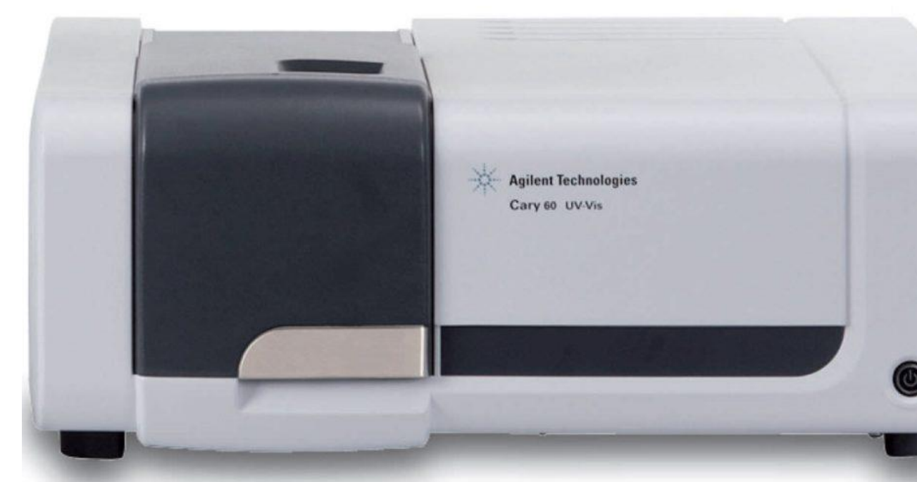
Fig. 5 Cary 60 UV-Vis is used as a Spectrophotometer. The laser in the machine measures absorbance at different wavelengths. This can be used to calculate the thickness of the sample.
