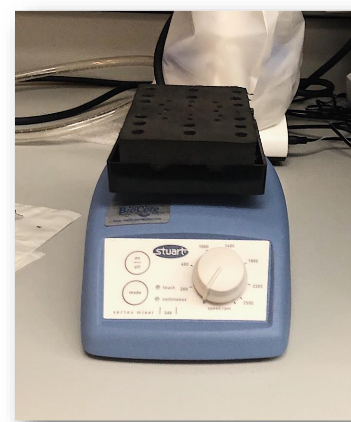
Fig. 3 Vortex Mixer is used to shake the polymer solution for the desired amount of time and speed (rpm).
